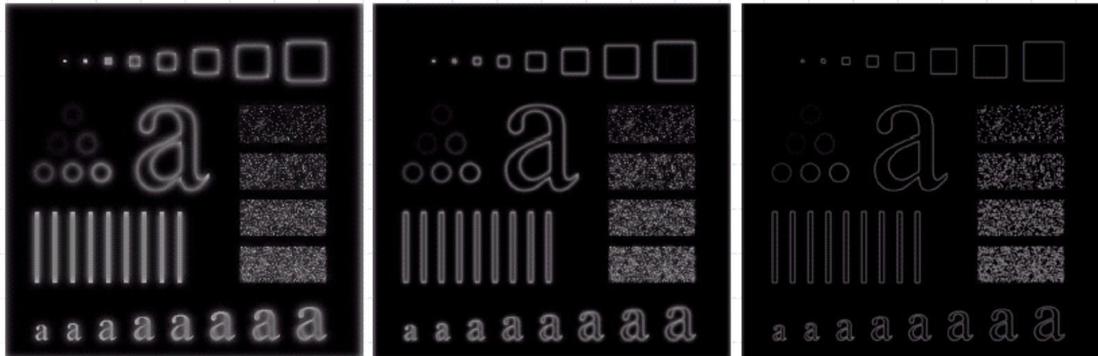
FIGURE 4.26 Results of highpass filtering the image of Fig. 4.11(a) using a GHPF of order 2 with D_0 = 15 , 30, and 80, respectively. Compare with Figs. 4.24 and 4.25.
